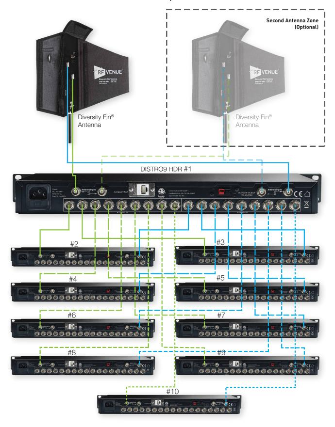
\*DISTRO9HDR #1 (Master) can feed signals to up to 9 additional DISTRO9HDRs. Each connected DISTRO9HDR can feed up to 9 receivers. \*Note: All outputs are equivalent. Any "A" can be paired with any "B" and any pair can be cascaded.
