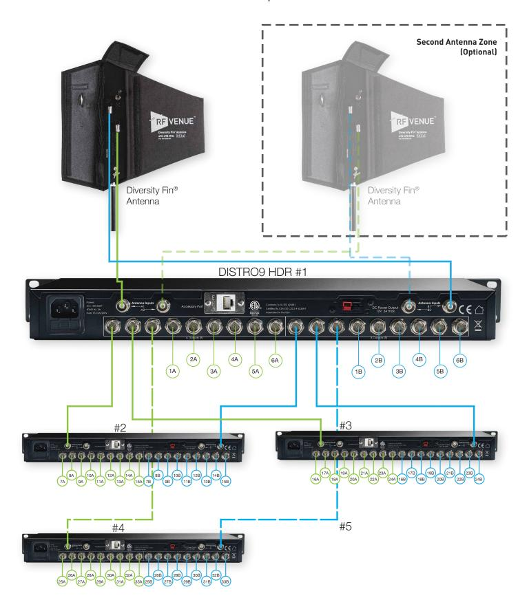
\*DISTRO9HDR #1 (Master) can feed signals to up to 9 additional DISTRO9HDRs. Each connected DISTRO9HDR can feed up to 9 receivers. \*Note: All outputs are equivalent. Any "A" can be paired with any "B" and any pair can be cascaded.
